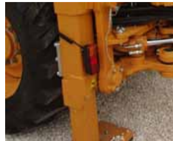
Rear road lights can be fitted on the stabiliser legs while travelling and on the cab when digging, providing maximum visibility and protection.
